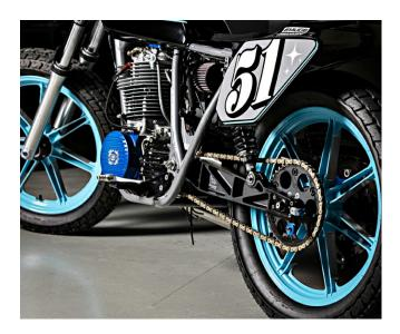
In the rear, two new shocks are attached to a custom swingarm – a part Maxime's boss requested to demonstrate the capabilities of Hurco's machine tools. The swingarm was made in collaboration with CAD/CAM company Mastercam and is custom-made for this bike. It features small details like a brake caliper support bracket and supports for a paddock stand.
