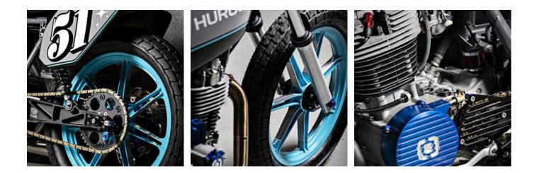
There is no brake at the front, but there is a Brembo caliper and master cylinder at the rear, connected by a stainless steel jacketed line. Since Maxime converted the bike from a rear drum brake, the entire brake system is custom – right down to the caliper mount and foot switches. Up front is a Yamaha XJR1200 suspension fork; the handlebar stem, triple clamps and handlebar risers are custom.
