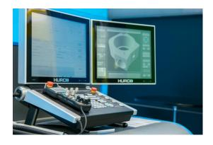
The 5-axis machines of the VMX series are equipped with the "WinMax" dialog control – optionally with DXF option. The powerful software of the control from HURCO simplifies programming for 5-sided machining and creates the conditions for the production of precision
