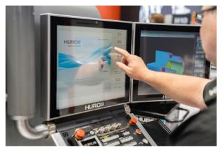
The programming time is reduced and simplified through simple data importing in the STEP 3D model format. The import option interprets the data and makes production programming directly at the machine possible. The path from workpiece to component becomes more secure as well. The potential for error during programming is reduced many times over, partly because the machining
