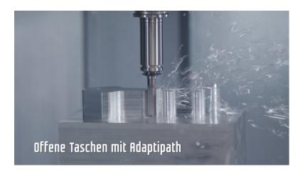
in a circular movement. Ideally, cutting takes place along the entire length of the cutter and the cutter is fully immersed in the workpiece.
