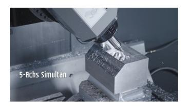
In the video we show the production of an engine block made of an aluminum alloy (AlCuMgPb) in a 5-axis machining we show the production of an engine block made of an aluminum alloy (AlCuMgPb) in a 5-axis machining. With this example, I would like to explain to you, among other things, the advantages of the  $AdaptiPath^{TM}$  option of our WinMax CNC control.
