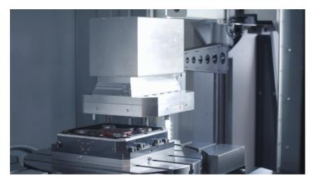
The automatic loading and unloading of the HURCO VMX 60 SRTi was carried out by the EROWA Robot Compact 80 pallet automation system from our Swiss cooperation partner EROWA. Here, the software of the ERC80 takes over and processes the production orders on the HURCO processing portal.
