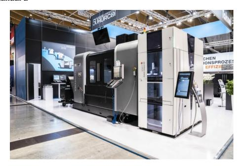
The foundations for rapid and application-oriented implementation of automation solutions, including digitalization, monitoring and evaluation, are contributed by a Windows-based operating system and the MT Connect open-source interface featured on HURCO assemblies. Network-supported DNC interfaces can be employed for mutual communications between
