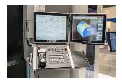
All HURCO machines are equipped with the "Max 5" conversational control system. Its high-performance WinMax CNC control software simplifies the programming. The control system is self-explanatory, ensuring that a short introduction is enough to cover the functionality. Trained employees are also quickly in a position to work with the control system. This greatly reduces the
