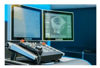
HURCO will be demonstrating just how easy programming with the Solid Model Import option at the AMB 2018 using several machine types as examples: 3D models that are available as STEP files can be imported directly with the new option. The import option interprets the data and enables production programming at the machine. This saves programming time and reduces the potential for errors during programming many
