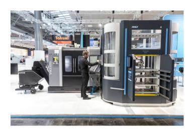
HURCO opted for the "Titanium" BMO system. This system allows a CNC machining center to be docked on both the left and right. Blanks are fed in the loading robot cell on trays. The robot arm integrated into the cell positions the blanks in the machining center, removes them after production and places them back into trays in the cell. "The operator loads the racks of the cell,
